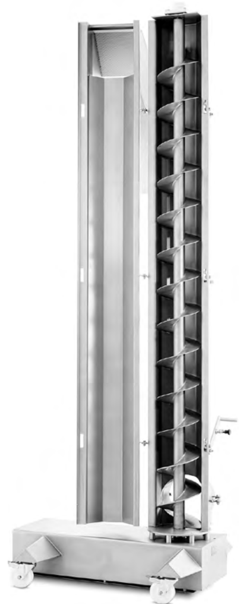
scansteel foodtech® standard scanGiraff, showing vertical screw.
