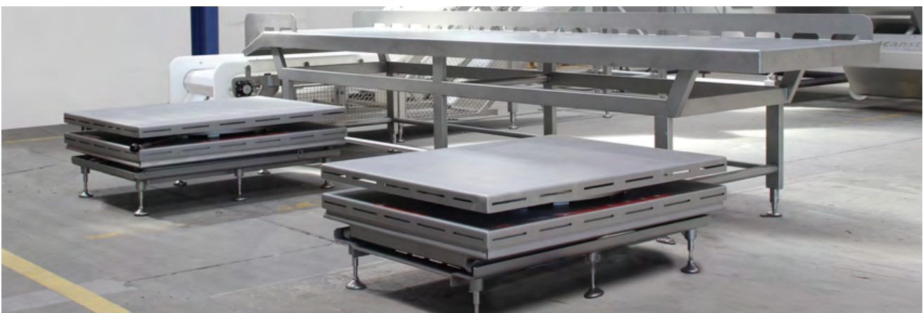
Unpacking station with 2 (two) lifting tables for ergonomics, right side.
