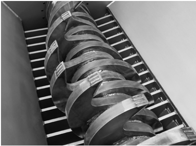
Crusher claw(s) made of mild steel with hard ended claw tips. Available dimensions of claw(s) for model A & B. (Cf page 5)
