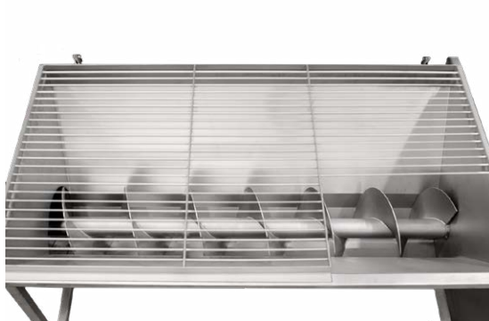
Infeed hopper shown with safety guard/grill in running position.
