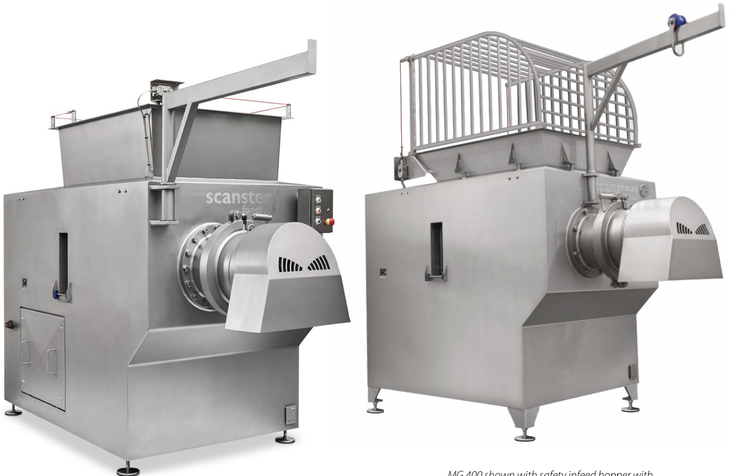
MG 400 shown with safety infeed hopper with trip wire.
